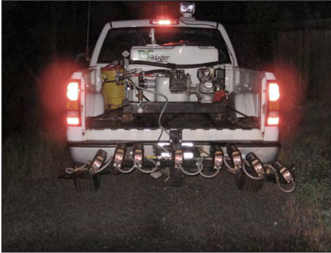
Photo a. Applying herbicide to gravel access road in early morning using a truck.
